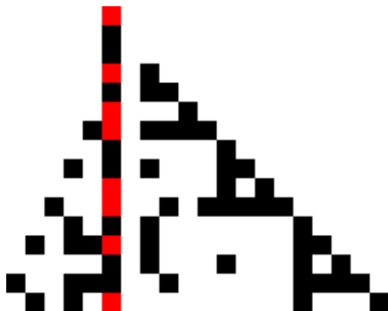
Figure : Spacetime diagram of a linear cellular automaton with memory 12 containing the Thue–Morse sequence as a column.
